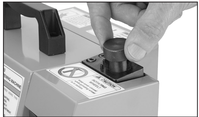
Figure 27. Cleaning rear trimming area.
